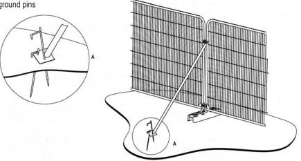
Figure 3b Stabiliser strut mounted on block tray
