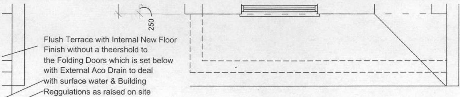
Flush Terrace with Internal New Floor Finish without a threshold to the Folding Doors which is set below with External Aco Drain to deal with surface water & Building Regulations as raised on site
