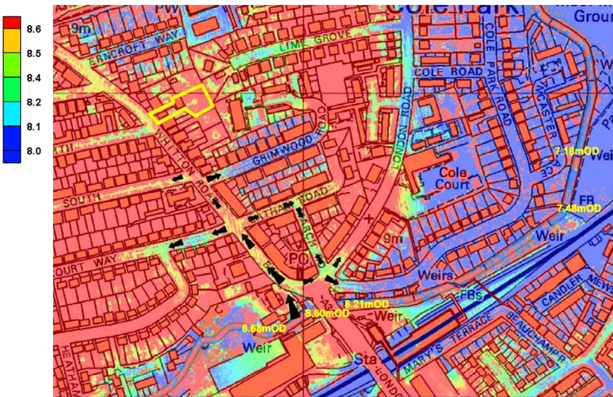
Figure 5.2 – DEM with potential flow paths marked on
